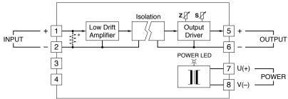
\*Input shunt resistor incorporated for current input.
