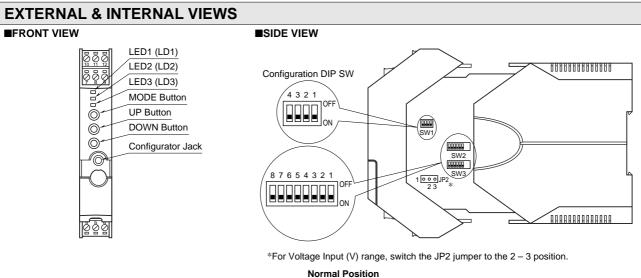
Normal Position (other than DC Voltage [V] range) DC Voltage [V] Range Position
